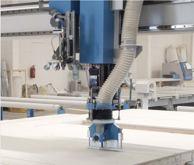
Saw unit ø 250 mm, HSK 63F with integrated extraction cover
