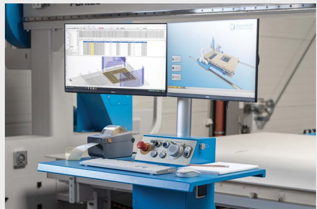
Integrated industrial PC Beckhoff with two large screen monitors; NCi control, TwinCAT 3
