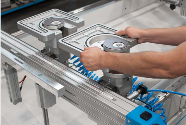
Vacuum pods with easy fixing for panel component production
