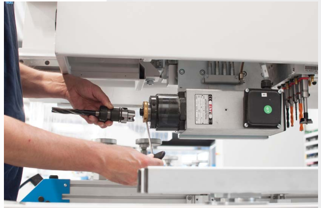
HSK 40A quick change system (horizontal milling unit)
