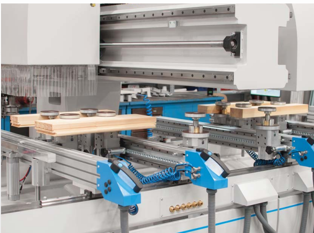
Clamping of 4 components at the same time
