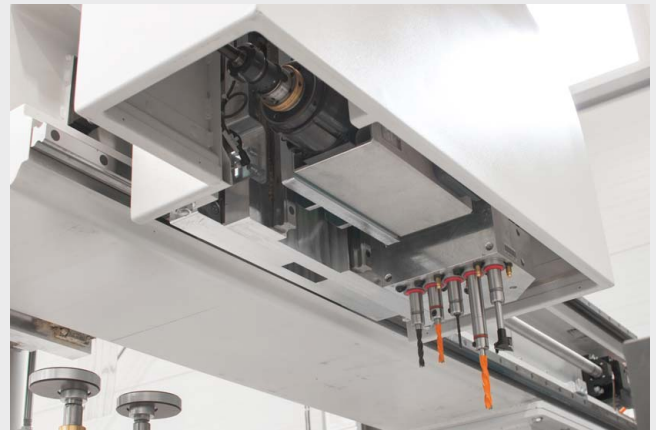
Vertical five spindle boring head and a horizontal milling unit with HSK 40A quick change system on the working axis Y-2
