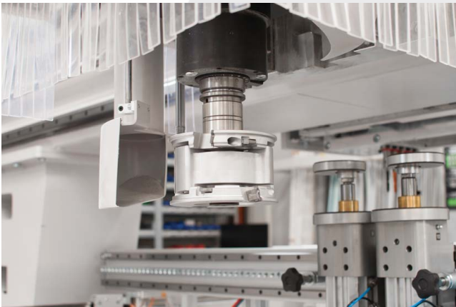
Vertical electro spindle HSK-F63 with C-Axis for aggregates on the working axis Y-1
