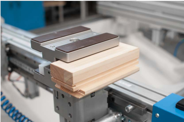
Special clamps for short components
