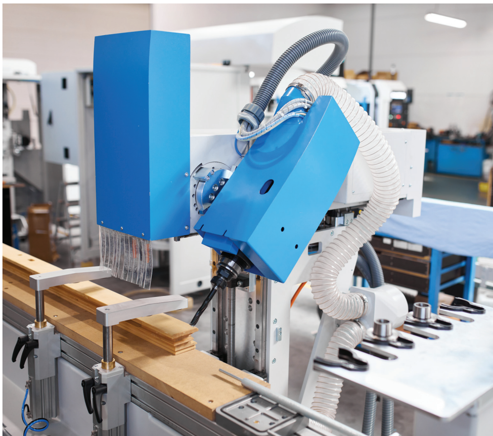
Main working units, tilting milling unit 0 - 90°
