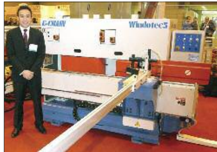
WindowTec5 from EChain - A sliding table movement is supported by an optional table movement that can be automatic with feed speeds of 5 to 20mtrs/min.
