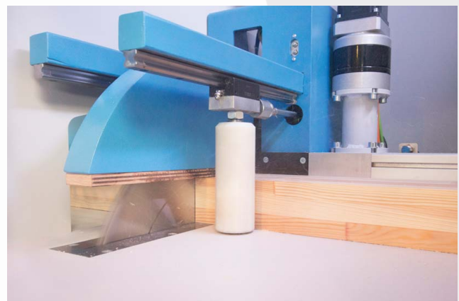
side and top clamp for precise cut
