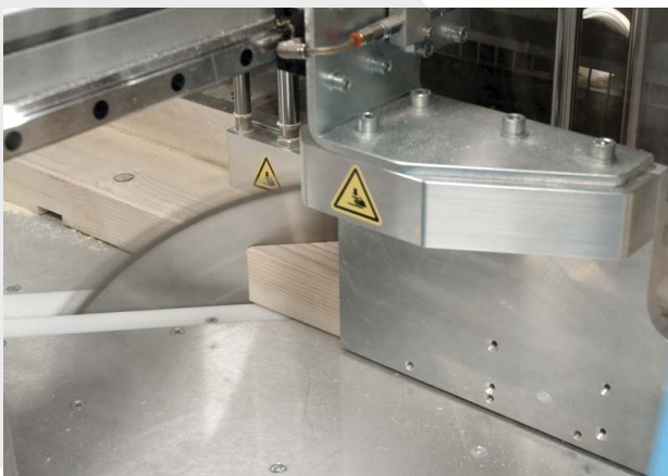
sawblade facilitating angled cuts
