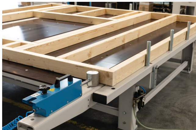
Pneumatic clamps with working force of 1200 N (6 bar)
