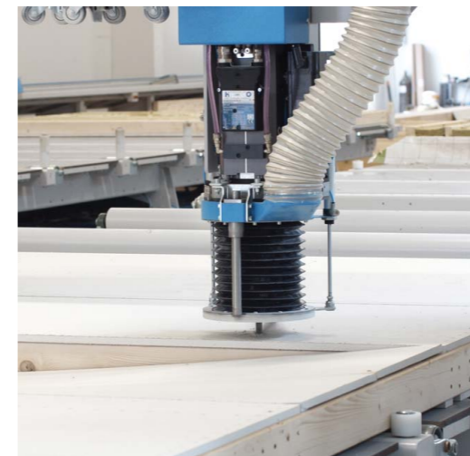
Saw unit with integrated extraction
