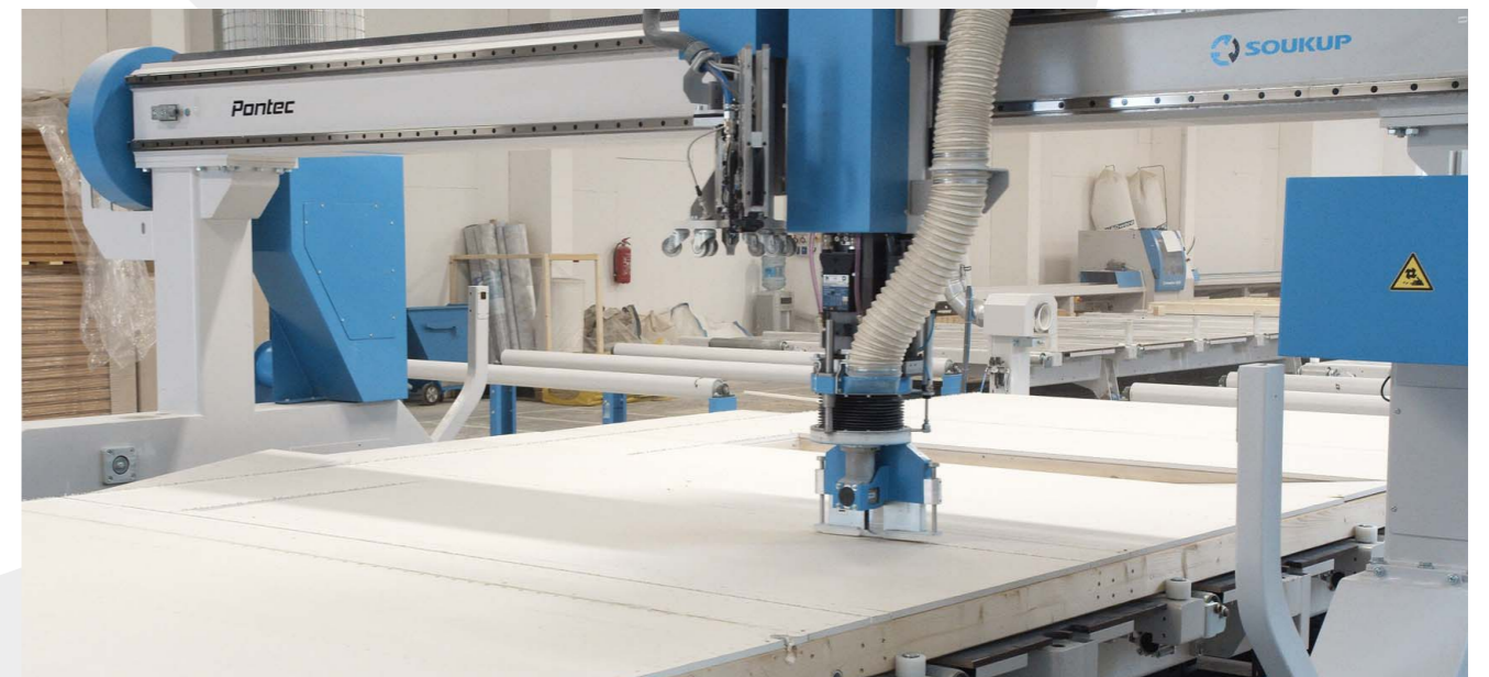
Saw unit with integrated extraction
